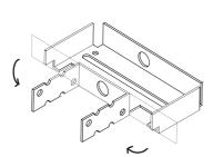
OPTIONAL: STEEL STUD ANCHOR 16 GA REINFORCEMENT CAN BE USE INSTED THE MULTI-PUPOSE ANCHOR.
